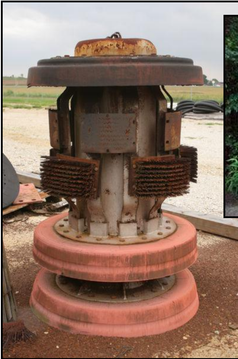
A pig used in natural gas pipelines
