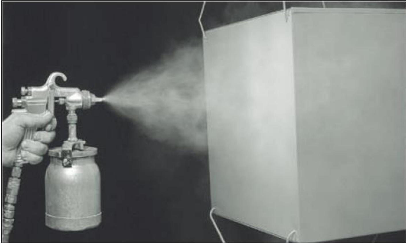
Fig.2: On external surfaces turbulent air spray creates excessive overspray and high material waste.
