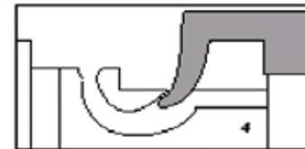
Runner defects at end of ejection
