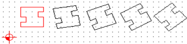
Fig. 15: For this example, the center of the contour was taken as reference point for the moving and the rotation. The rotating angle is 10^\circ and the number of copies 4.
